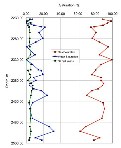
**Figure 20.** Illustrates fluid saturation (gas, oil, and water) of the Montney Formation from well 16-17-82-25W6, northeastern British Columbia (Data source: B.C. Oil and Gas Commission).
