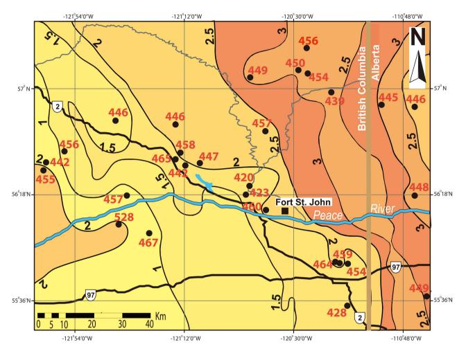
**Figure 13.** The Montney Formation average Tmax (°C) map. Tmax values are posted over TOC map to show geographical distribution of source rock quality (TOC), and thermal maturity of source rock. The red dots represent wells with Rock-Eval data. Evidently, the Montney Formation kerogen is thermally matured, and it is within the "peak gas" generation window in the study area, northeastern British Columbia, and northwestern Alberta as shown by the average Tmax values.
