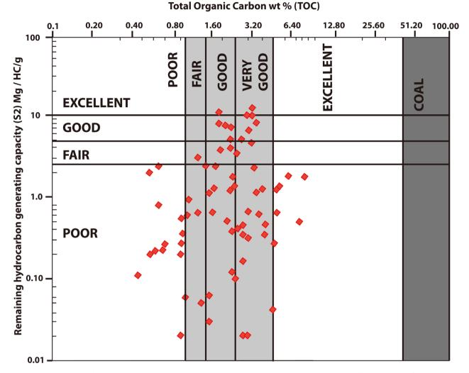
**Figure 21.** A cross plot showing total organic carbon (TOC wt%) values and S2 values (the amount of hydrocarbon formed during thermal decomposition of kerogen). The higher S2 values indicate greater hydrocarbon generating potential. In general, the S2 and TOC values show that the Montney Formation in the study area, northeastern British Columbia has good source rock quality. However, some of the data points also indicates poor to fair.
