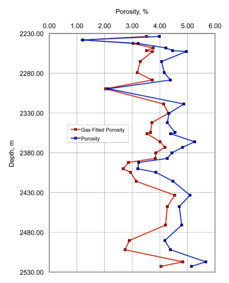
**Figure 16.** Shows porosity and gas filled porosity of the Montney Formation (well 16-17-82-25W6). The graph shows very excellent correlation between porosity and gas filled porosity. (Data source: B.C. Oil and Gas Commission).
