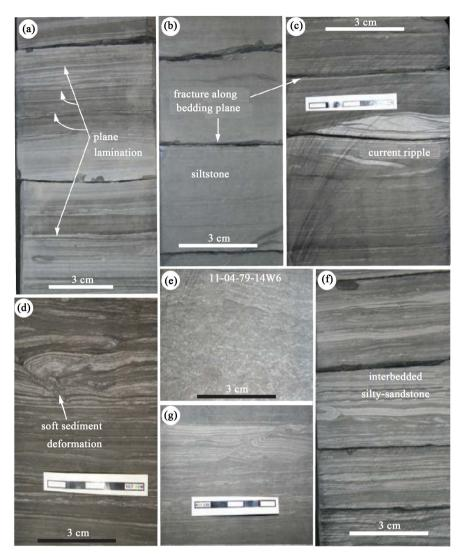
**Figure 5.** Shows lithofacies of the Montney Formation (a) Plane lamination; (b) fractured siltstone along bedding plane; (c) silty-sandstone with current ripple sedimentary structure; (d) shows sediment deformation structure; (e) bioturbation by *Phycosyphon?*; (f) interbedded silty-sandstone.
