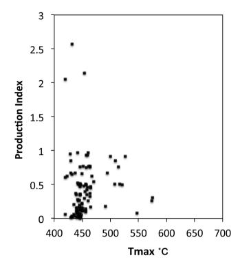
Figure 15. Shows that the Montney Formation kerogen is thermally matured, and extensively composed of gas.
