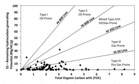
**Figure 11.** Shows S2 peak (remaining hydrocarbon generating capacity) for the Montney Formation, which corresponds to the Tmax. The S1 peak is the liberated hydrocarbon during rapid artificial thermal cracking of kerogen during pyrolysis (see **Figure 10**). Sample location: well 2-19-79-14W6 (depth: 2085 m).
