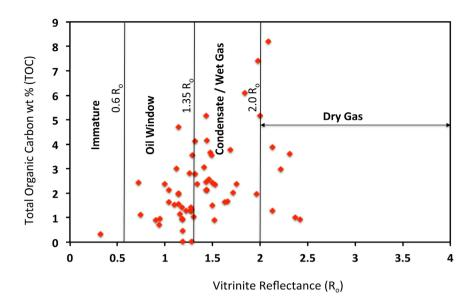
**Figure 14.** Total Organic carbon (TOC) vs. vitrinite reflectance ( $R_o$ ) showing the thermal maturity of Montney Formation source-rock, and hydrocarbon generating phases in the Montney Formation sediments from study area, northeastern British Columbia [24].
