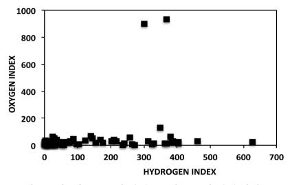
**Figure 8**. Shows a plot of Oxygen Index (OI) vs. Hydrogen Index (HI). The low OI and HI indicate that the Montney Formation in the study area is primarily a Type III/IV kerogen, with a mixed Type II/III kerogen.
