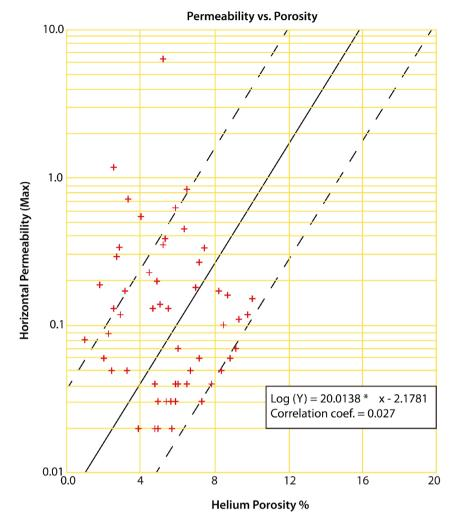
**Figure 17.** Porosity vs. permeability crossplot for the Montney Formation, well: 2-19-79-14W6 (depth 2037.40 - 2091.90 m). Data source: B.C. Oil and Gas Commission.
