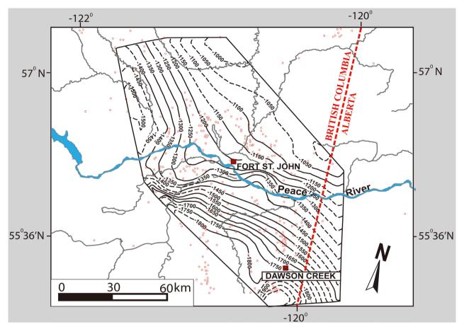
**Figure 3.** Structure contour map of the Montney Formation in the study area, northeastern British Columbia. Dash contour lines indicate no data point for well control. The structure map decreases in elevation westward, which indicates that sediment source area was from east, and prograded westward [2].
