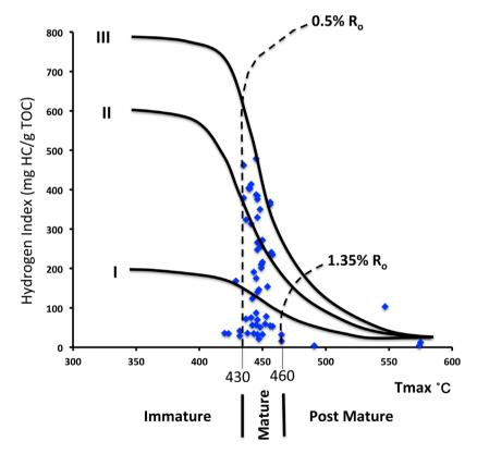
**Figure 12.** Thermal maturity of the Montney Formation determined with Tmax and vitrinite reflectance (Ro). The dotted line (Ro) is vitrinite reflectance calibrated with Tmax. This shows that the Montney Formation in northeastern British Columbia is extensively matured [24].
