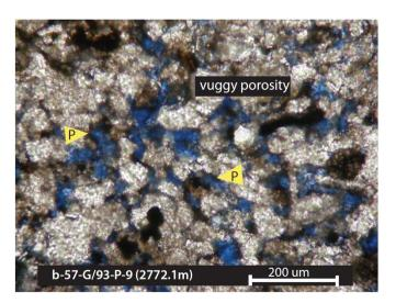
**Figure 18.** Microphotograph showing dolomitic siltstone facies and the associated vuggy porosity resulting from dissolution of material. Yellow arrow labeled "P" is pointing to vuggy porosity.
