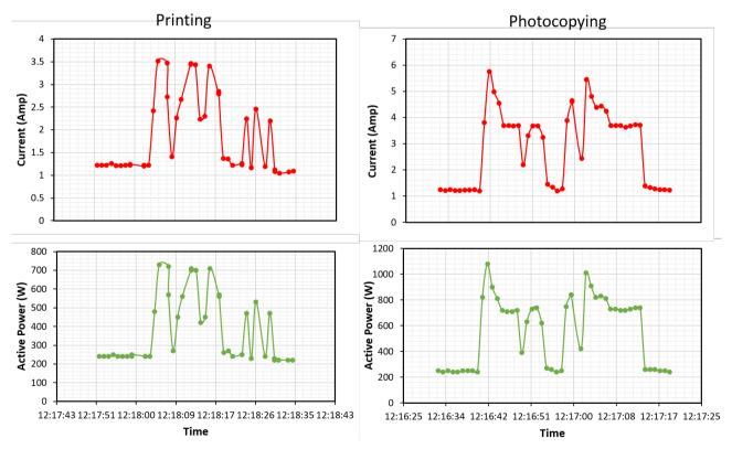
Figure 9. Comparison of current and active power for printing and photocopying.
