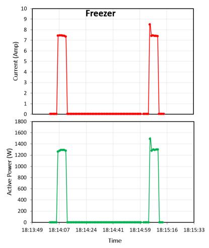
Figure 7. Current and active power for a freezer.
