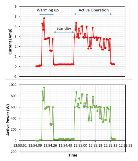
Figure 10. Current and active power for a photocopy machine.
