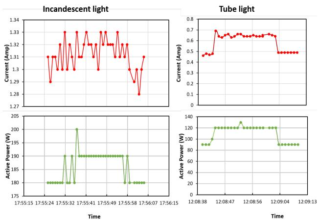
Figure 4. Current and active power for lights.
