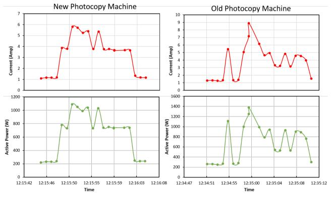
Figure 6. Current and active power for the photocopy machines.
