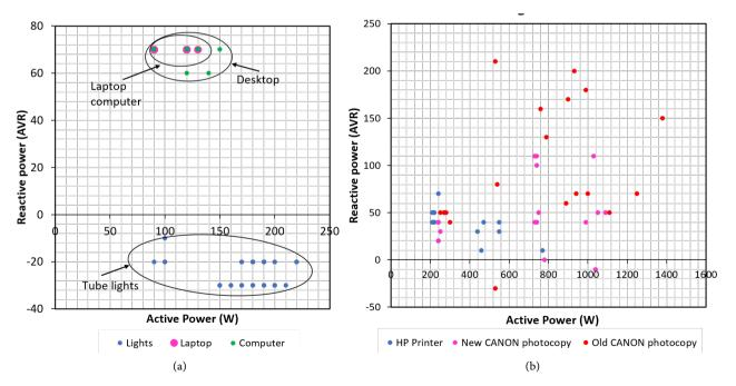
Figure 8. Active and reactive power of electric loads in administration block.
