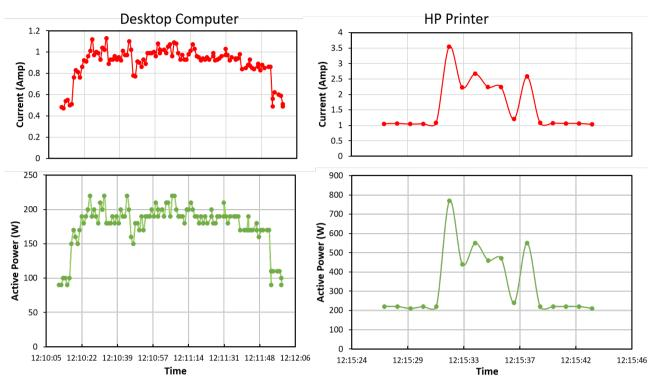
Figure 5. Current and active power for desktop computer and HP printer.
