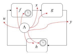
Figure 1. Generalized cyber attacks on a typical NCS.
