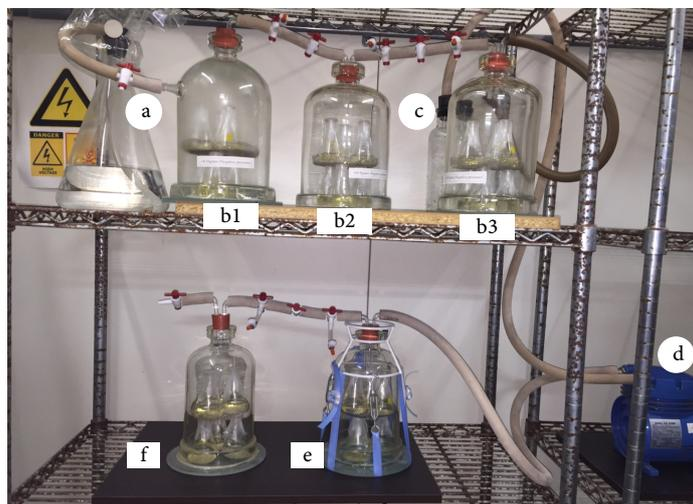
**Figure 1.** (a) Humidifier unit; (b) Hypobaric chambers: (b1)  $-50$  mmHg, (b2)  $-100$  mmHg, (b3)  $-150$  mmHg; (c) Pressure stabilizer; (d) Air pump; (e) Hyperbaric ( $50$  mmHg); (f) Control.
