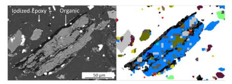
**Figure 1.** BSE image of a Kupferschiefer particle (left) and in MLA false colours (right) showing detection of organic matter and successful differentiation from the iodized epoxy resin. (MLA colours: black/ dark grey: organic matter, blue: sheet silicates, green: carbonates, light grey: quartz, red/ violet: copper sulphides).
