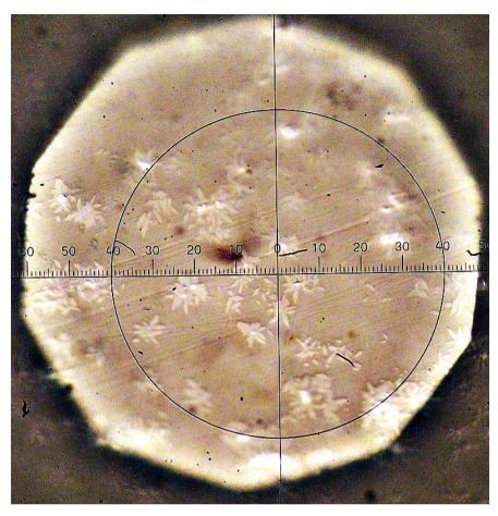
Figure 13. Optical photo of crystals of magnesiochromite (white centers) and diopside of outlet in glass I a. Thermal history: 740°C 4 h - for the nucleation of magnesiochromite and 750°C for 4 h + 880°C 20 min - for the nucleation and development of diopside. Graduation is 1 µ.
