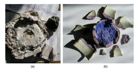
**Figure 1.** The appearance of the linings of cooking stoves (a) and security of the crucible (b) after melting slag I.
