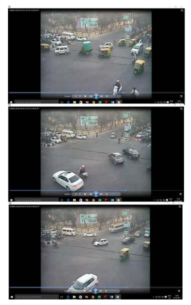
**Figure 3.** Traffic data collection for a typical junction by videography.
