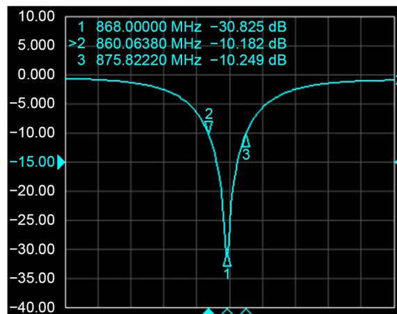
Figure 13. Measured reflection coefficient of the proposed PIFA.
