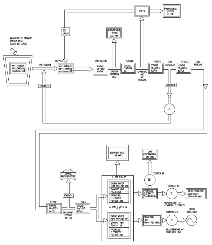
Figure 2. Diagram of the plant and the fuel flow.
