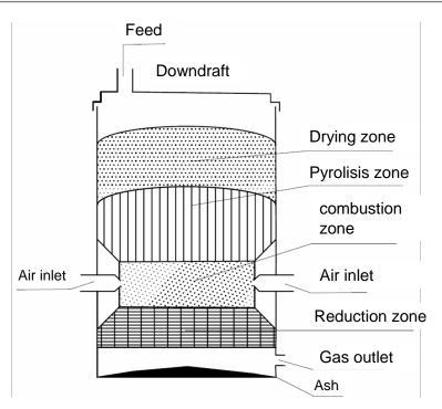
Figure 3. Downdraft gasifier diagram.
