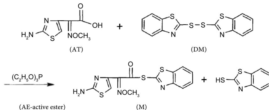
**Figure 2.** Synthetic route of AE-active ester.
