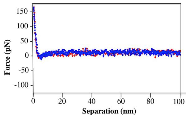
**Figure 7.** Typical F-D curves of AFM tips modified with lysine on mica surface. Red and blue traces indicate signals upon approach and retraction from surface, respectively.
