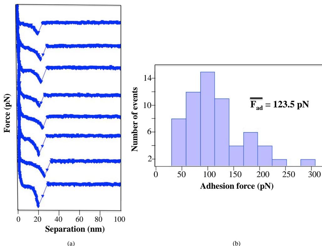
**Figure 6.** (a) Typical F-D curves during retraction of an AFM tip modified with lysine on pyrite are displayed vertically. These force curves were produced from three different functionalized tips with the same loading rate of 6 nN/s; (b) Unbinding force histogram. MPF for lysine on pyrite surface at loading rate of 6 nN/s (pH = 7.4). Average adhesion force was calculated by using Gaussian fit and shows mean of 123.5 pN.
