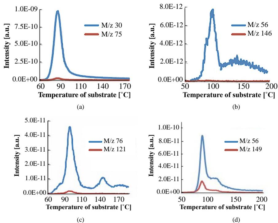
**Figure 9.** TDS spectra of (a) glycine; (b) lysine; (c) cysteine; and (d) methionine on pyrite (pH = 7.4). First and second peaks indicate the physisorption and chemisorption, respectively.
