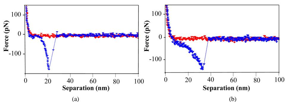
**Figure 8.** Specific adhesion force curve of an AFM tip modified with (a) methionine and (b) cysteine on pyrite surfaces. The red and blue traces indicate the signal upon approach and retraction from the surface, respectively.
