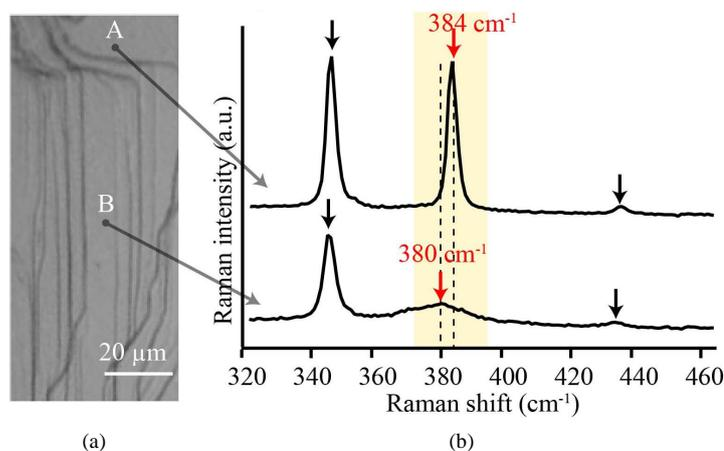
**Figure 4.** (a) Optical microscope image of outer surface of pyrite; (b) Raman spectra of pyrite outer surface measured at positions A and B. Considerable differences between the two spectra, particularly in terms of the frequencies, intensities, and widths of their  $A_g$  mode peaks, are observed.
