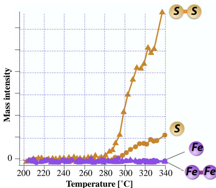
**Figure S1.** TDS spectra of sulfur-monomer ( $m/z$  32) and sulfur-dimer ( $m/z$  64) with temperature change of natural pyrite in vacuum. Sulfur-dimer peak is much higher than monomer peak. No significant desorption is observed for irons.
