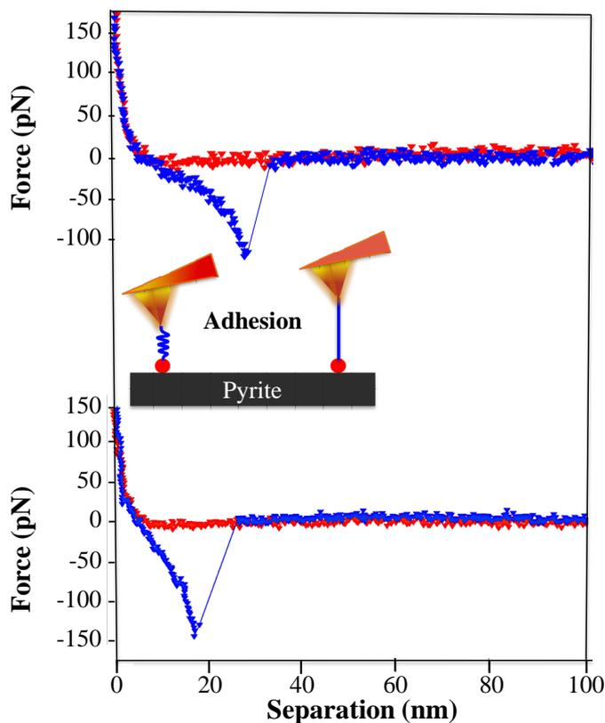
**Figure 5.** Force measurement between lysine and pyrite. Typical single-molecule F-D curves of AFM tip modified with lysine on pyrite surface. Specific adhesion events are evident during AFM probe retraction; Red and blue traces indicate signals upon approach and retraction from surface, respectively.
