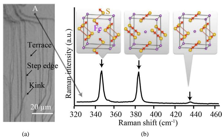
**Figure 3.** (a) Optical microscope image of outer surface of pyrite. Step edge, terrace, and kink on the sample surface are marked by arrows; (b) Raman spectra of pyrite outer surface indicated by point A in the optical image.
