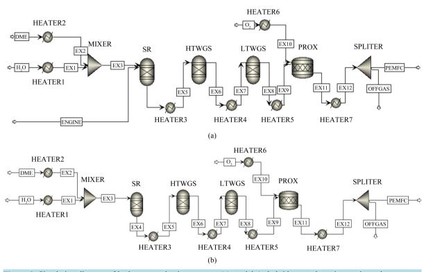
Figure 2. Simulation diagram of hydrogen production process: (a) model A: hybrid power by using engine exhaust gas as heat source, (b) model B: using reactor as heat source.
