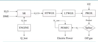
Figure 1. Flowchart of hydrogen production system.
