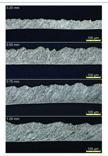
Figure 11. Microphotograph of chips obtained by changing the depth of cut.
