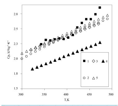
Figure 1. Comparison of the experimental and calculated heat capacity values of the oil (Sample No.1): 1—experiment; 2—calculation according to [73]; 3—calculation according to [65]-[67]; 4—calculation according to [52].
