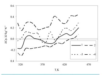
**Figure 7.** Excess heat capacity of the oil and oil-products: 1—oil (sample No.1); 2—deasphaltizate; 3—asphalt; 4—bitumen.
