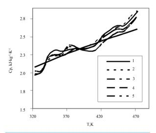
Figure 6. Heat capacity of the oil (sample No.2) at various pressures: 1 - P = 0.098 MPa; 2 - P = 9.8 MPa; 3 - P = 19.6 MPa; 4 - P = 29.4 MPa; 5-calculation according to [65]-[67].
