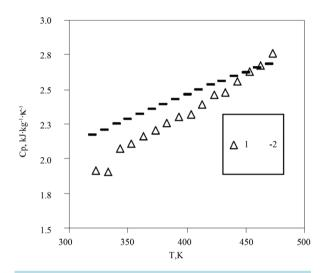
**Figure 3.** Heat capacity of deasphaltizate: 1—experiment; 2—calculation according to [65]-[67].
