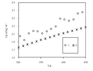
Figure 4. Heat capacity of asphalt: 1—experiment; 2—calculation according to [65]-[67].
