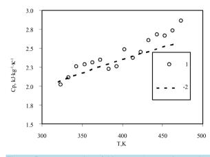
Figure 5. Heat capacity of bitumen: 1—experiment; 2– calculation according to [65]-[67].
