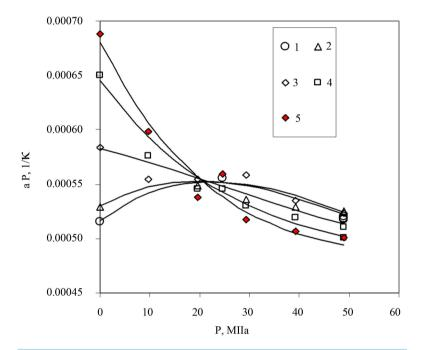
**Figure 9.** Pressure dependence of the thermal expansion coefficient at various temperatures *T*, K (continues lines-smoothed-out data, dots-experiment): 1-T = 298 K; 2-T = 303 K; 3-T = 323 K; 4-T = 348 K; 5-T = 363 K.
