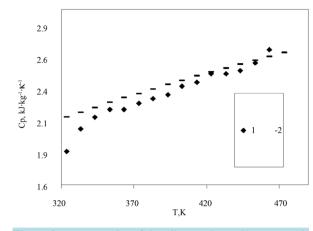
Figure 2. Heat capacity of the oil (sample No.2): 1—experiment; 2—calculation according to [65]-[67].
