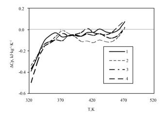
Figure 8. Excess heat capacity of the oil (sample No.2) at various pressures: 1-P = 0.098 MPa; 2-P = 9.8 MPa; 3-P = 19.6 MPa; 4-P = 29.4 MPa.
