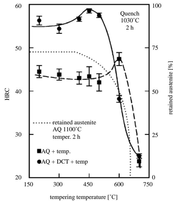
**Figure 7.** Influence of deep cryogenic treatment on hardness of X30CrMoN15-1 (quenching at 1150°C).
