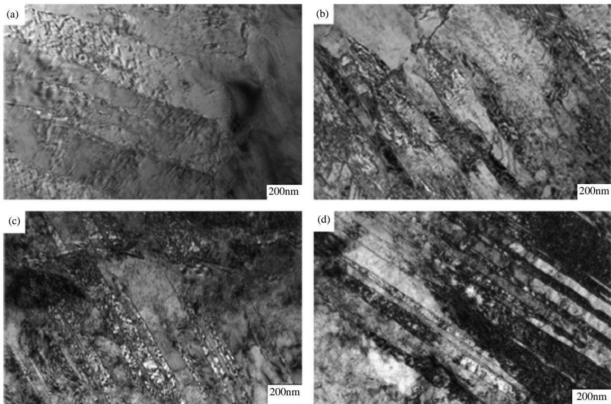
**Figure 3.** TEM morphology of specimens at different cryogenic treatment. (a) Treatment C; (b) Treatment D; (c) Treatment E; (d) Treatment F.
