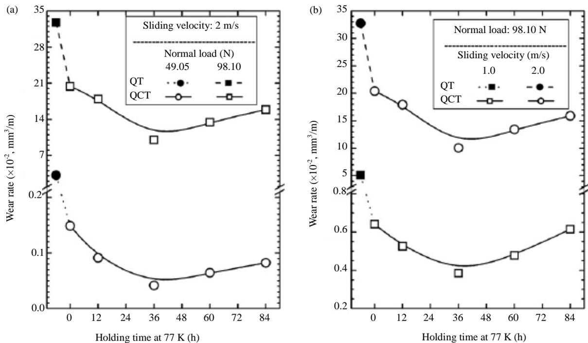
**Figure 13.** A remarkable benefit on antiwear ability of D2 die steel through cryogenic treatment.
