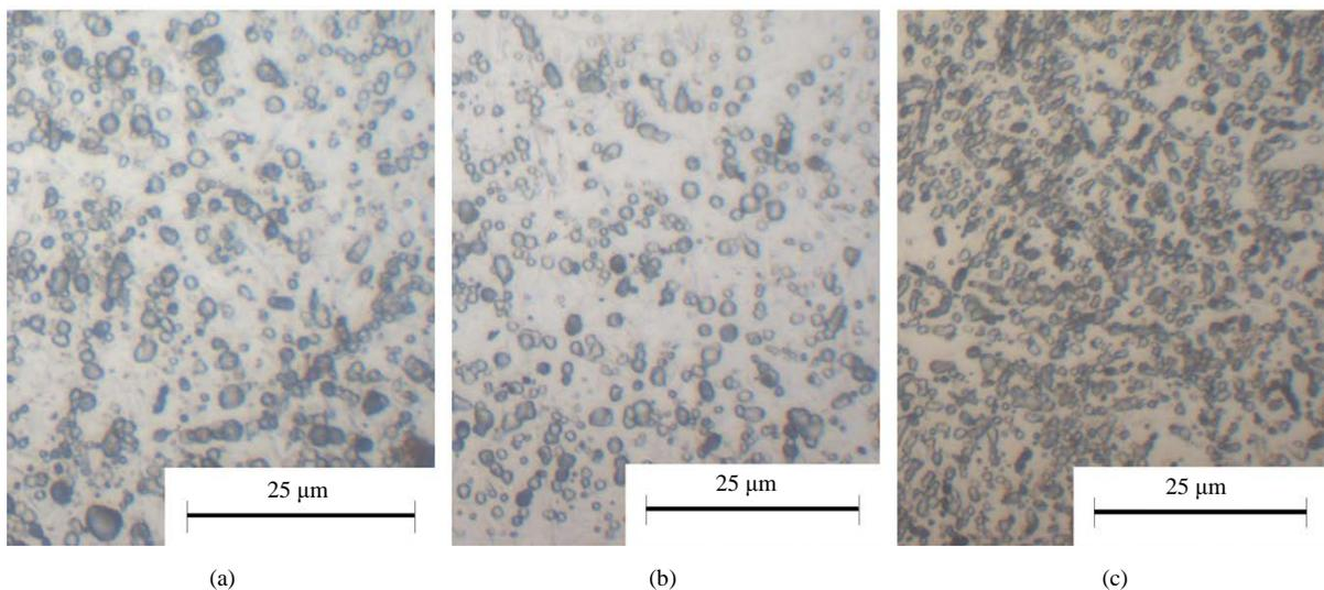
**Figure 2.** Quenching microstructure of 30CrMoN15-1: martensite + carbide. (a) Water quenching at  $1000^{\circ}\text{C}$ ; (b) Water quenching at  $900^{\circ}\text{C}$ ; (c) Air quenching at  $1000^{\circ}\text{C}$ .
