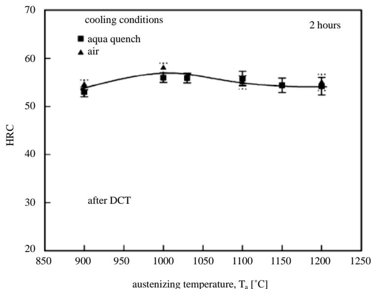
**Figure 5.** Hardness of X30CrMoN15-1 maintains constant when a deep cryogenic treatment follows after quenching.
