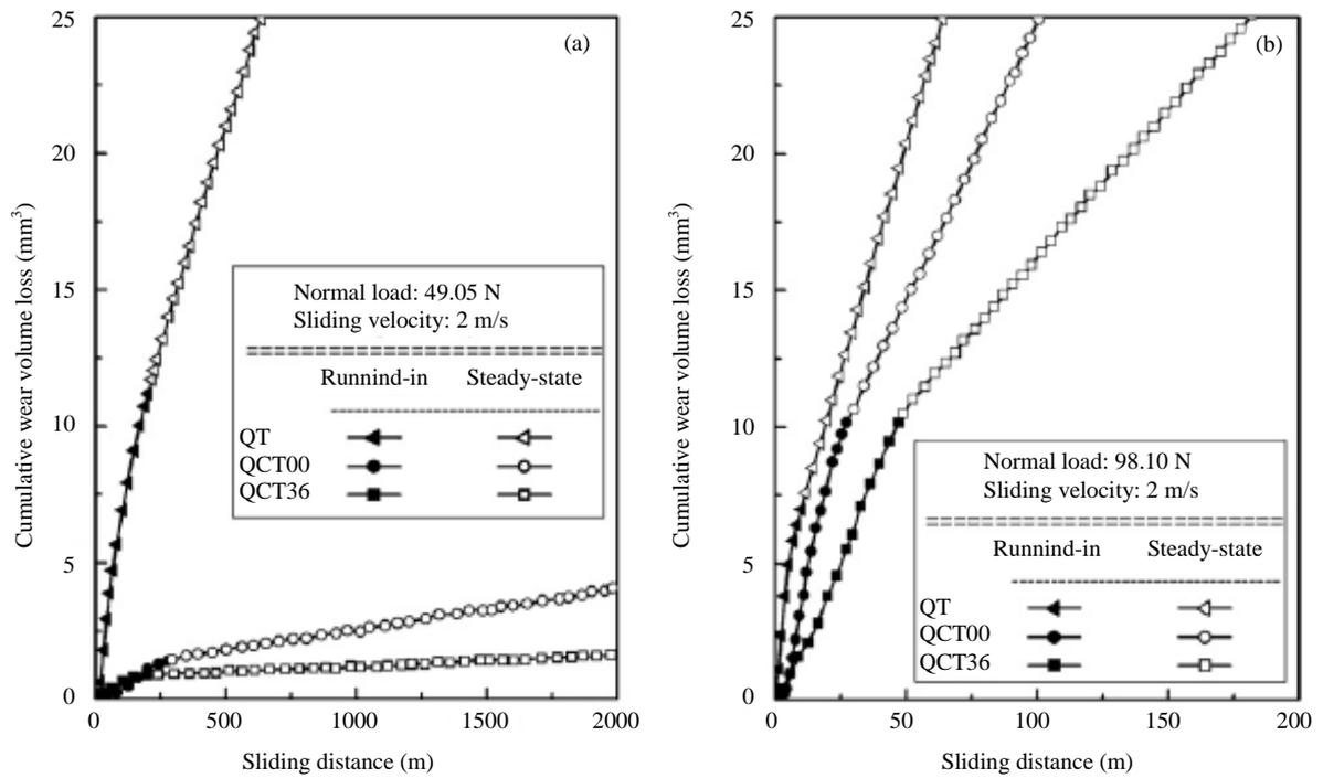
**Figure 12.** The correlation between sliding distance and accumulative wear volume.
