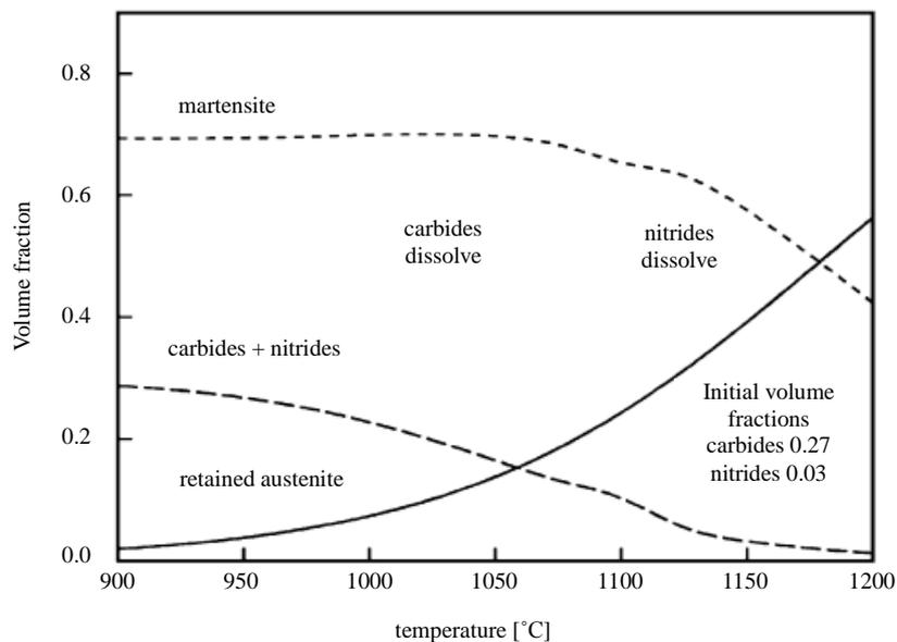
**Figure 8.** Function relevance between microstructure ingredients of X30CrMoN15-1 and quenching temperatures with deep cryogenic treatment following after quenching.
