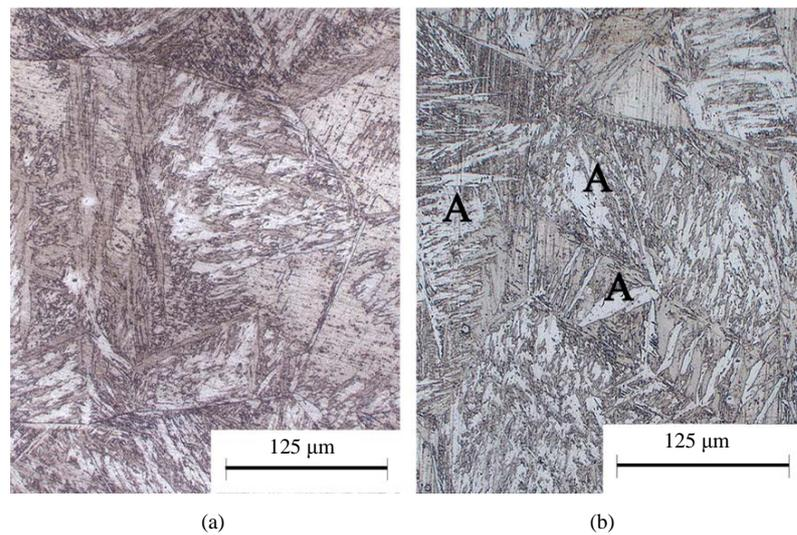
**Figure 1.** Quenching microstructure of 30CrMoN15-1: martensite + carbide + retained austenite. (a) Quenching in ethylene glycol at  $1200^{\circ}\text{C}$ ; (b) Quenching in air at  $1200^{\circ}\text{C}$ .
