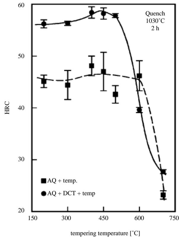
**Figure 6.** Influence of deep cryogenic treatment on hardness of X30CrMoN15-1 (quenching at 1030°C).
