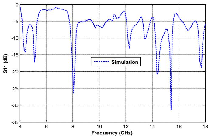
Figure 6. Variation of return loss with frequency for the proposed antenna.
