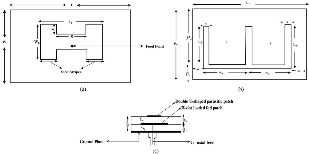
**Figure 1.** Configuration of stacked patch antenna. (a) H-slot loaded fed patch; (b) Double U-shaped slots loaded parasitic patch; (c) Side view of the proposed antenna.
