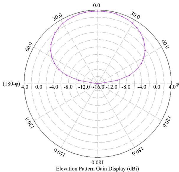
Figure 8. Radiation pattern of the proposed antenna at frequency 8.08 GHz.
