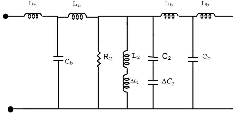
**Figure 4.** Equivalent circuit of U-slot loaded patch.
