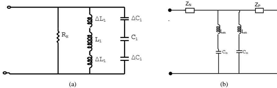
**Figure 3.** (a) Equivalent circuit of RMSA due to notch effect; (b) Equivalent circuit of H-shaped fed patch.
