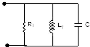
Figure 2. Equivalent circuit of patch antenna.
