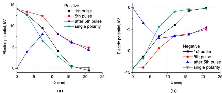
**Figure 8.** Typical distribution of the electric potential over the surface for the 1<sup>st</sup> pulse in the burst, at the 5<sup>th</sup> pulse, after the 5<sup>th</sup> pulse, and for a single polarity at the 8<sup>th</sup> pulse. (a) Positive polarity; (b) Negative polarity.
