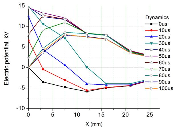
**Figure 9.** Dynamics of the X-distribution of the surface potential during and after the  $\tau = 50 \mu\text{s}$  positive pulse following the negative pulse,  $U_{\text{max}} = 15 \text{ kV}$ .
