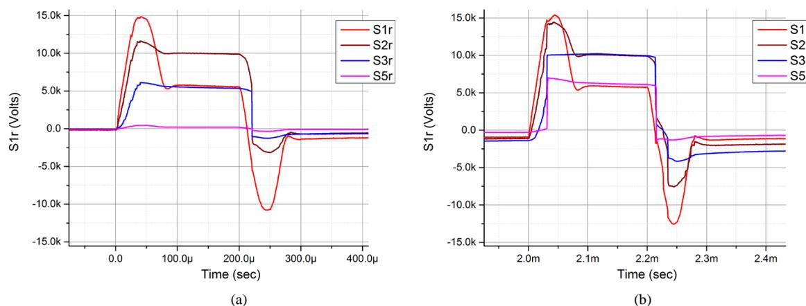
**Figure 6.** The surface electric potential dynamics depending on the pulse number, detail view. (a) The first positive and negative pulses; (b) The 8<sup>th</sup> positive and negative pulses.
