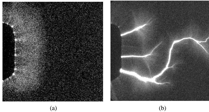
**Figure 4.** ISSD camera images of the SDBD in diffusive (a) and contraction (b) mode. Negative polarity, first pulse in the burst.
