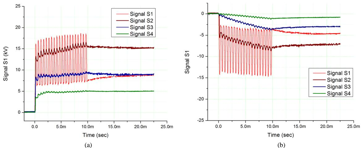
**Figure 3.** Surface charge sensors typical traces. S1-S4—sensor numbers from closest to exposed electrode to the furthest away. (a) Positive polarity; (b) Negative polarity.
