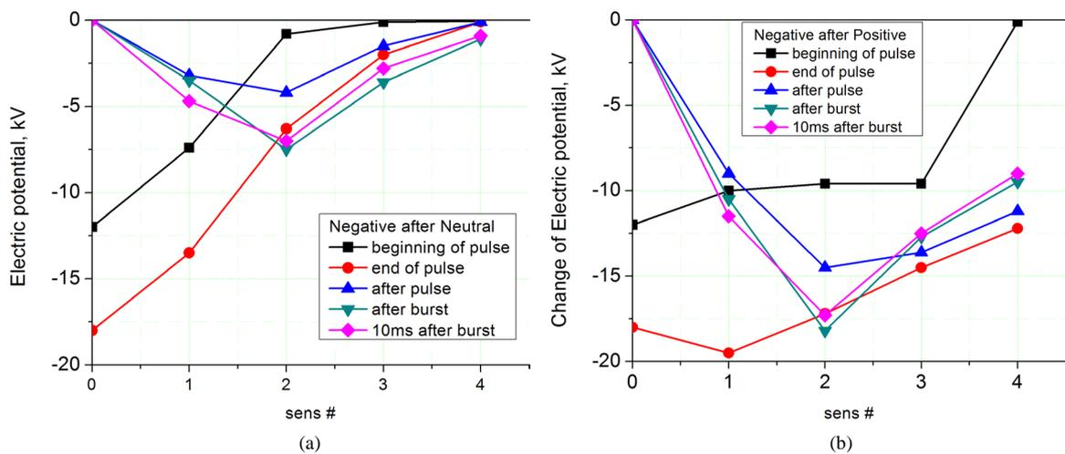
**Figure 5.** Electric potential distribution over the surface at and after the negative pulses. (a) No discharge contraction; (b) Discharge contraction observed.
