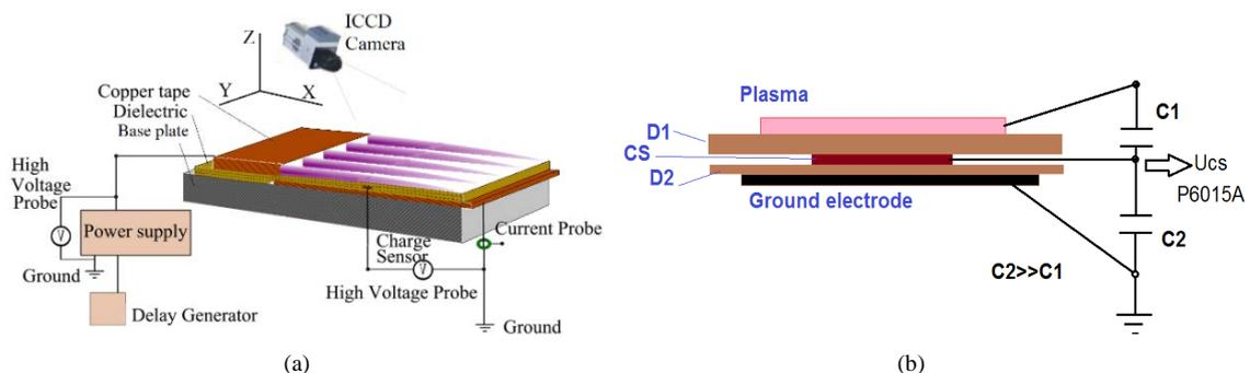
**Figure 1.** Experimental test cell layout (a); Scheme of the charge sensor assembly (b).
