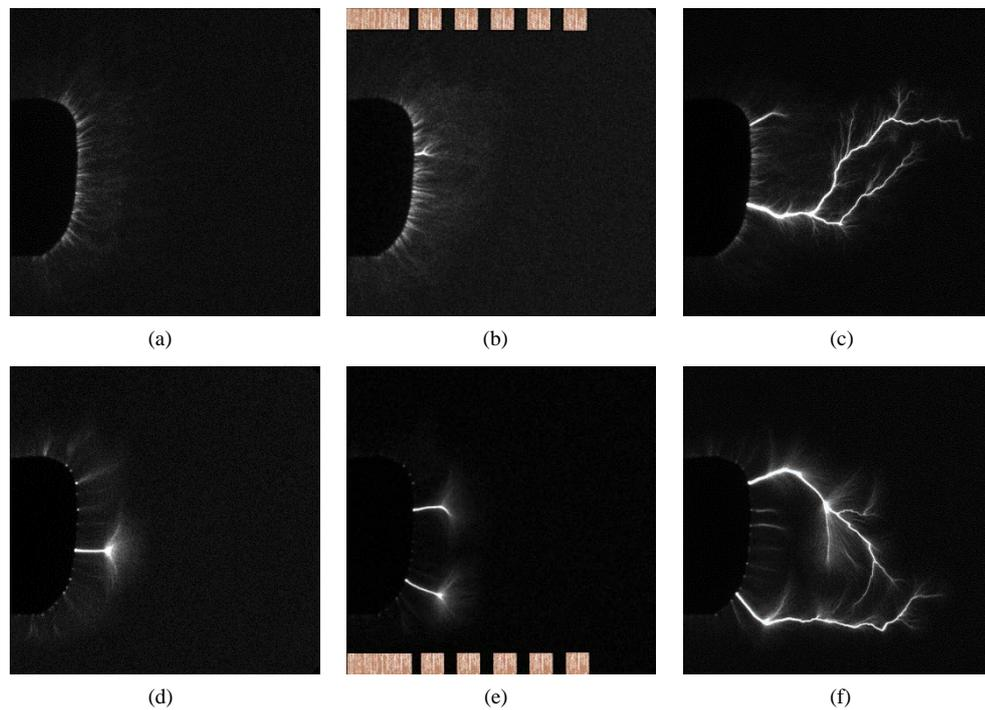
**Figure 7.** Discharge images, taken sequentially in the burst. Top row ((a)-(c)) positive polarity; bottom row ((d)-(f)) negative polarity. The pulse pair number is #1 ((a) and (d)), #2 ((b) and (e)), and #8 ((c) and (f)). The HV electrode and CS positions are indicated by insertion in (b) and (e) images.
