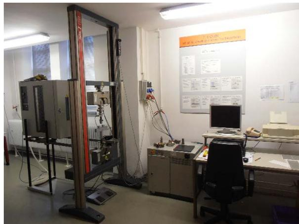
**Figure 3.** Bending Test Equipment (Zwick Machine, PC).
