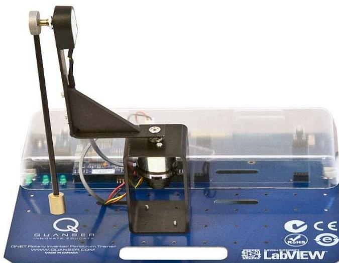
**Figure 1.** The quaser inverted pendulum system.
