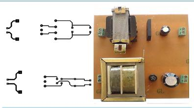
Figure 12. Printed circuit of supply circuit.
