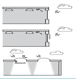
Figure 6. Positioning of lux sensor in the laboratory.
