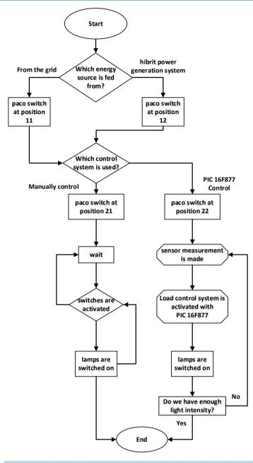
Figure 8. Flow diagram of load control system.
