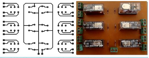
Figure 9. Printed circuit of disconnector circuit and completed situation of component mountings.
