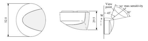
Figure 5. General view of lux sensor and field of vision of lux sensor.
