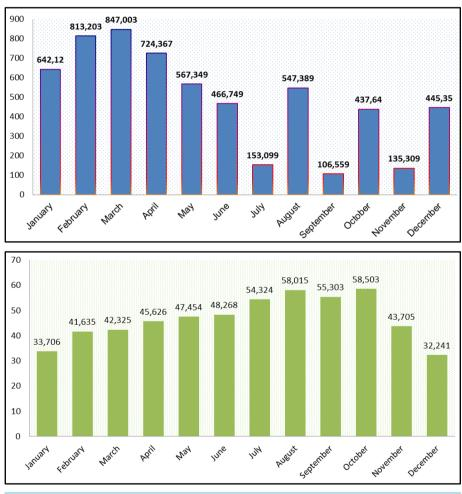
Figure 13. Energy generated by wind turbine and solar panel by months (Wh).
