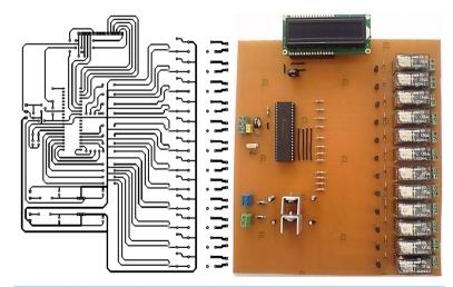
Figure 11. Printed circuit schema of the load control circuit that is transferred on plaque and of which component mounting has been made.
