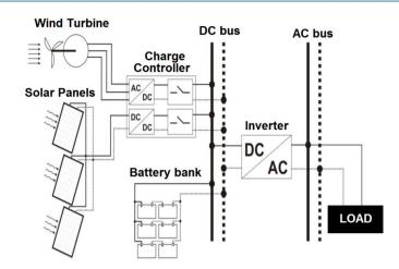
Figure 1. General view and open connection schema of battery-aided wind-solar hybrid power generation system.
