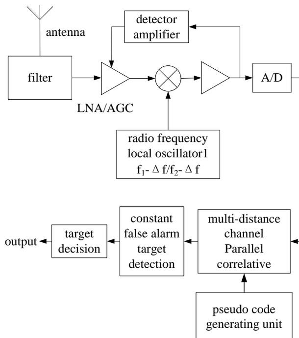
**Figure 3.** The receiving module of rangefinder.
