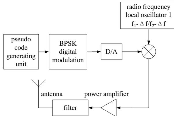
**Figure 2.** The sending module of rangefinder.
