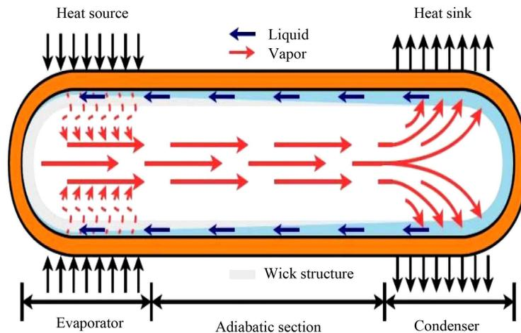
**Figure 1.** Schematic of a heat pipe.
