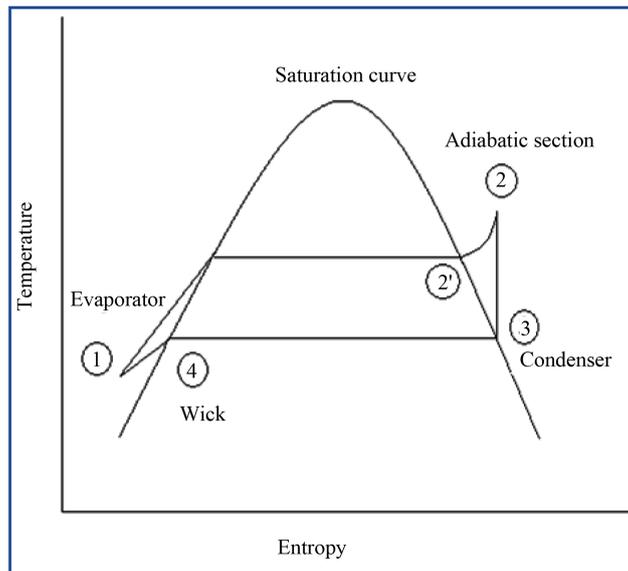
**Figure 4.** Thermodynamic operation of heat pipe.
