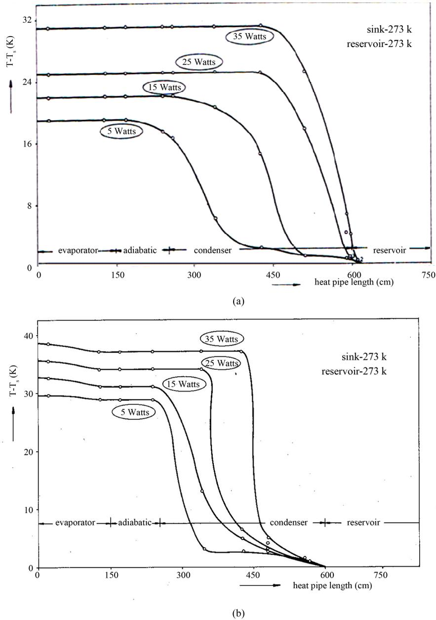
**Figure 7.** Wall Temperature along methanol VCHP with Control gas (a) NH<sub>3</sub>, (b) N<sub>2</sub>, [30].
