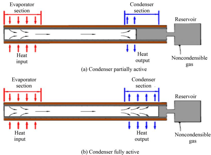
**Figure 6.** Variable conductance heat pipe.
