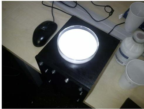
**Figure 12.** Measurement of Intralipid in a petri dish with Dermalog spectrometer.
