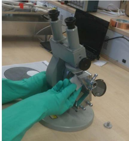
**Figure 27.** Measuring the refractive index of the phantom at the Abbé refractometer.
