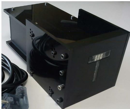
**Figure 5.** Demonstration of the Dermalog spectrometer with light source and the entrance slit.
