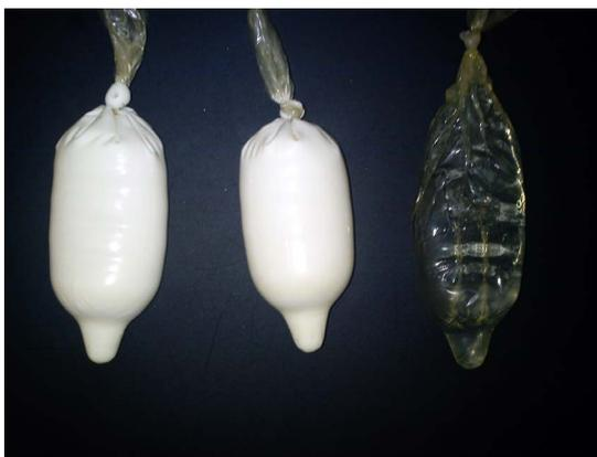
**Figure 15.** Latex sheaths with Intralipid-water mixtures.
