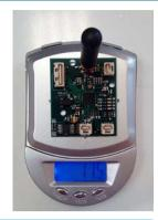
Figure 1. Size (a little larger than a 2 € coin) on the left and weight (less than 12 g) of the latest version of RFID tags on the right, without the equipment to recharge it and without battery.
