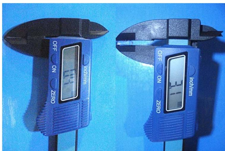
**Figure 2.** The pachymeter for determining the thickness of GG2% hydrogel in dried and swollen form.
