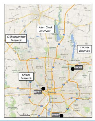
Figure 1. Reservoirs that contribute to the Columbus, Ohio water supply are Griggs, O'Shaughnessy, Alum Creek, and Hoover. The Dublin Road Water Plant (DRWP) extracts water from Griggs and O'Shaughnessy for water supply usage, while the Hap Cremean Water Plant (HCWP) utilizes water from Hoover Reservoir. Alum Creek Reservoir provides supplemental water to Hap Cremean Water Plant (adapted from Google maps). Parsons Avenue Water Plant (PAWP) distributes groundwater from wells.
