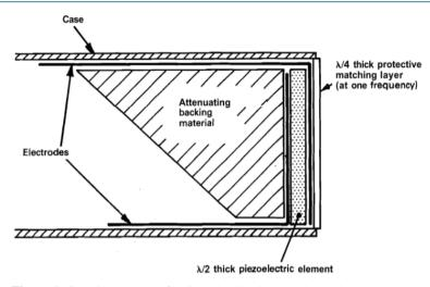
Figure 1. Generic structure of a piezoelectric ultrasound transducer [1].
