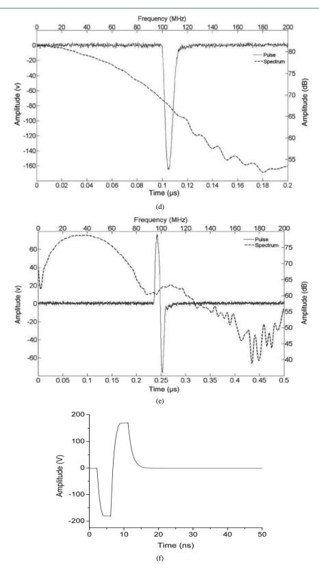
**Figure 7.** Outputs of pulse generators involved in this Paper: (a) Circuit designed in this paper; (b) Output in [2]; (c) Output in [3]; ((d), (e)) Unipolar and bipolar output in [4]; (f) Bipolar output in [5].
