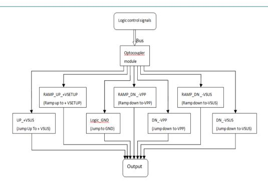
Figure 2. The schematic block diagram of the circuit design.
