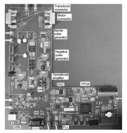
Figure 8. PCB board provided in [4].
