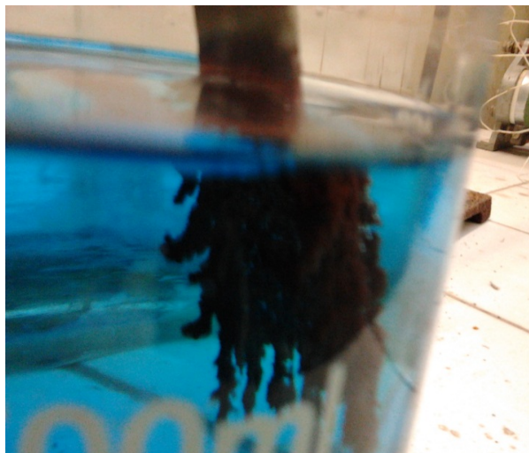
Figure 10. Deposition of copper powder on cathode showing massive dendrites.
