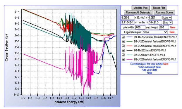
Figure 1. Fission and neutron capture rates for uranium and thorium
