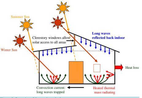
Figure 5. Operation of the passive solar house.
