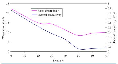
Figure 1. Variation of thermal conductivity and water absorption at 25°C.
