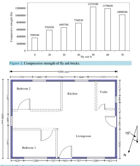
Figure 3. The floor plan of the passive solar house.
