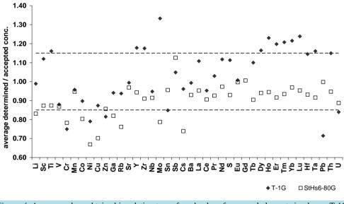
**Figure 4.** Average values obtained in relation to preferred values for several elements in glasses T-IG (quartz diorite) and StHs6/80G (andesite), compared with the mean certified values cited in [17], cf. **Table 10** and **Table 11**.
