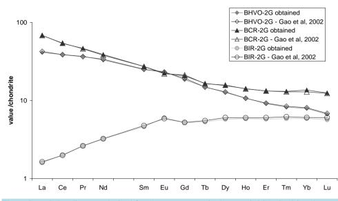
Figure 2. Variation diagrams obtained for the REE contents in the BHVO-2G, BCR-2G and BIR-1G basaltic glasses, normalized with C1 chondrite [16] [17].
