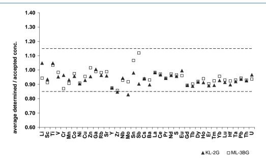
Figure 3. Average values obtained in relation to preferred values for several elements in basalt glasses KL-2G and ML-3BG, compared with the mean values cited in [17], cf. Table 8 and Table 9.
