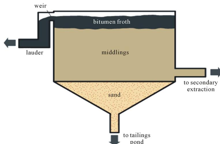
**Figure 4.** Diagram of a conventional primary separation vessel (PSV).
