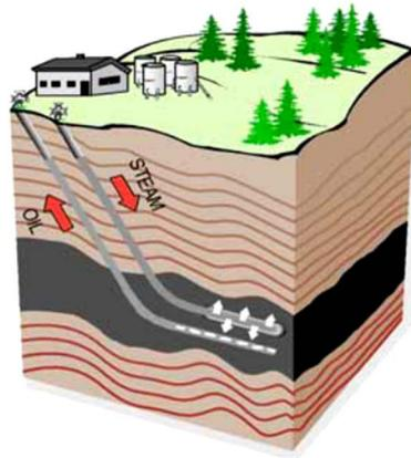
**Figure 3.** Steam assisted gravity drainage method of *in situ* processing.
