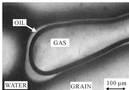
**Figure 5.** Image of an oil-coated bubble for oil-assisted flotation [16].
