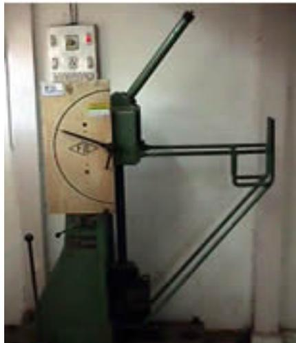
Figure 5. Impact testing machine.
