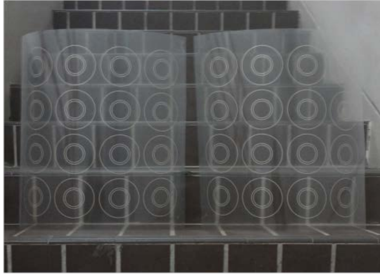
Figure 8. Photo of the fabricated flexible and transparent tri-band rejection EMI shield.
