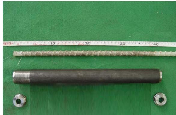
Figure 3. Steel adapter of FRP Hybrid Bars for tensile test.
