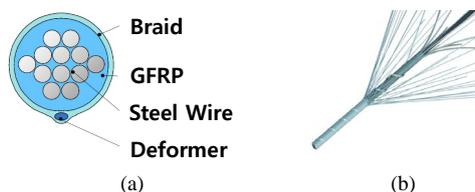
**Figure 1.** Schematic details of cross section (a) and configuration of manufacturing processes (b) for FRP Hybrid Bars.
