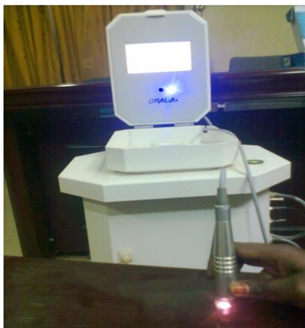
**Figure 2.** Irradiation of specimens by diode laser (810 nm).
