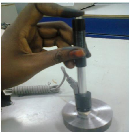
**Figure 3.** The method of hardness measured.
