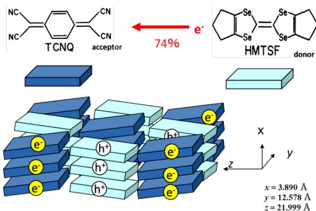
**Figure 2.** Schematic view of the crystal model of HMTSF-TCNQ. Both HMTSF and TCNQ molecules stack themselves along the 1D-axis. Since the axis indexing for  $a$ ,  $b$  and  $c$  is different among the bibliography, to avoid confusion, we adopt the naming of  $x$ ,  $y$  and  $z$  axes for the most conducting to the least conducting axes.
