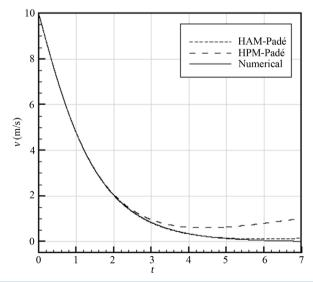
**Figure 3.** The velocity in  $\theta$  direction for water with r = 0.01,  $\omega = 1000$  rad/s,  $v = 1.519 \times 10^{-6}$  (m<sup>2</sup>/s),  $\rho = 1000$  (kg/m<sup>3</sup>).
