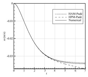
Figure 4. The velocity in z direction for water with r = 0.01,  $\omega = 1000 \text{ rad/s}$ ,  $v = 1.519 \times 10^{-6} \text{ (m}^2/\text{s)}$ ,  $\rho = 1000 \text{ (kg/m}^3)$ .
