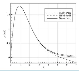
**Figure 2.** The velocity in r direction for water with r = 0.01,  $\omega = 1000$  rad/s,  $v = 1.519 \times 10^{-6}$  (m<sup>2</sup>/s),  $\rho = 1000$  (kg/m<sup>3</sup>).
