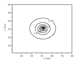
Figure 5. Protection zone of a lightning rod at Z = 15 m, L = 20 m.
