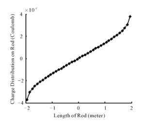
Figure 2. Charge distribution on the lightning rod, L = 4 m.
