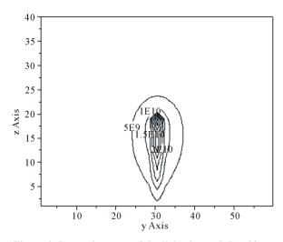
Figure 3. Protection zone of the lightning rod, L = 20 m.
