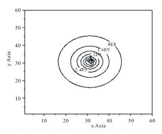
Figure 4. Protection zone of the lightning rod at Z = 5 m, L = 20 m.
