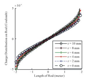
Figure 6. Charge Distribution on the lightning rod L = 4 meter.
