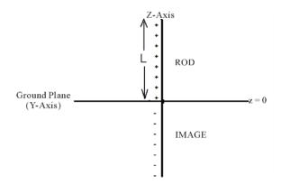
Figure 1. Lightning rod modeled as a 1-dimensional structure.
