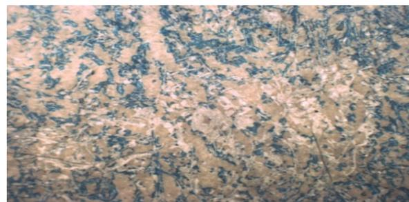
**Figure 13.** Photomicrograph of offset prints on paper coated with clay coating mixture containing MA/AA 30:70 binder. At Magnification  $\approx 4\times$ .
