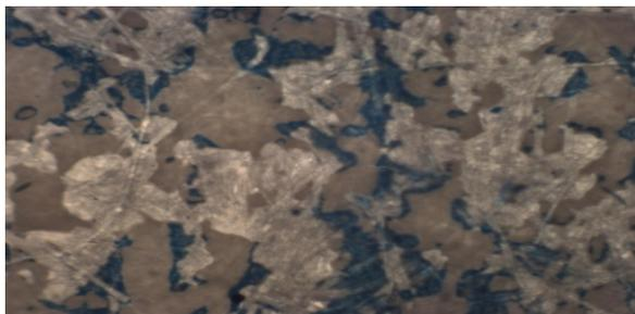
**Figure 10.** Photomicrograph of offset prints on paper coated with clay coating mixture containing MA/AA 70:30 binder. At Magnification  $\approx 10\times$ .
