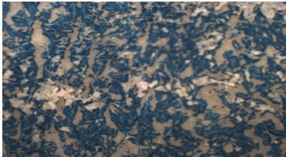
**Figure 8.** Photomicrograph of offset prints on paper coated with clay coating mixture containing MA/AA 90:10 binder. At Magnification  $\approx 4\times$ .
