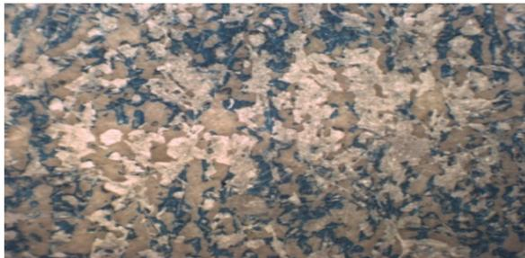
**Figure 9.** Photomicrograph of offset prints on paper coated with clay coating mixture containing MA/AA 70:30 binder. At Magnification  $\approx 4\times$ .
