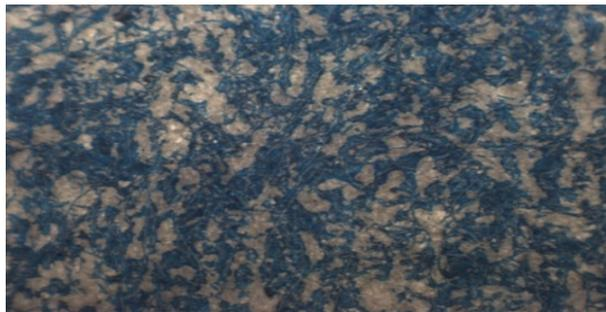
**Figure 17.** Photomicrograph of offset prints on paper coated with clay coating mixture containing (MA/AA + AMPS/AA) blend binder. At Magnification  $\approx 4\times$ .
