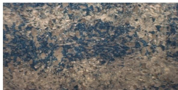
**Figure 14.** Photomicrograph of offset prints on paper coated with clay coating mixture containing MA/AA 10:90 binder. At Magnification  $\approx 4\times$ .
