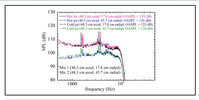
Figure 3. Narrowband acoustic spectrum for cold and hot jets for microphones 1 and 2.
