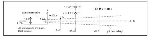
Figure 1. Schematic of the experimental configuration and microphone setup.
