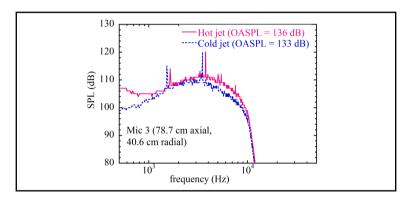
Figure 4. Narrowband acoustic spectrum for cold and hot jets for microphone 3.
