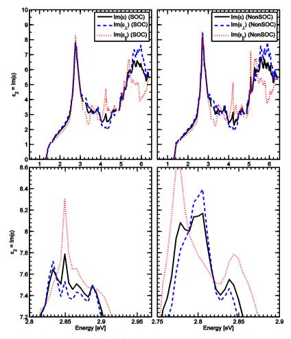
Figure 3. The tensor of complex of the dielectric function is presented (left and right panel). The average of the polarization along the x and y directions is  $\varepsilon_{\perp}$  and parallel with the z direction is  $\varepsilon_{\parallel}$ . The main peak is presented in the lower panel.
