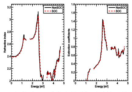
Figure 5. The average real and imaginary part of refractive index (left panel and right panel) is shown.
