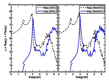
Figure 2. The average of complex of dielectric function is presented (left and right panel).  $\operatorname{Re}(\varepsilon)$  is the real part of the dielectric function, and  $\operatorname{Im}(\varepsilon)$  is the imaginary part of dielectric function.
