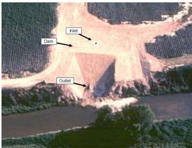
**Figure 1.** Aerial photograph of newly installed drop pipe structure.
