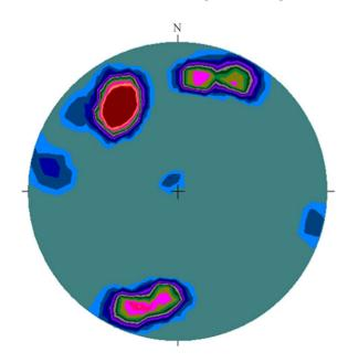
Figure 5. Contoured poles of fractures in the sandstone of Ségou area lower hemisphere equal angle projections.
