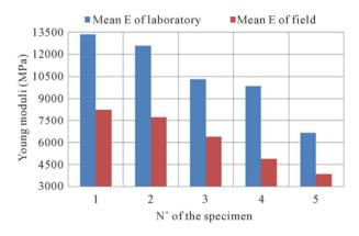
Figure 6. Graphical representation of Young moduli for different kind of basalts in laboratory samples and field ones (1: healthy basalts, 2: basalts with unfilled fractures, 3: basalts with tension cracks filled with quartz, 4: basalts with multiple fractures, 5: basalts with fractures filled with calcite, chlorite, epidote).
