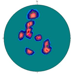
Figure 3. Contoured poles of fractures in the basalts (lower hemisphere equal angle projections): cylindrical folds southwest of Bafoundou.
