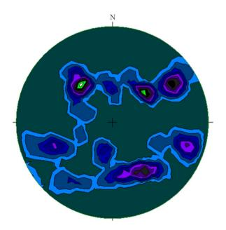
Figure 2. Contoured poles of fractures in the basalts (lower hemisphere equal angle projections): conic folds in the Mako area.
