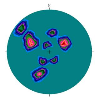
Figure 4. Contoured poles of fractures in the basalts (lower hemisphere equal angle projections): superposed cylindrical and conic fold.
