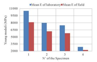
Figure 7. Graphical representation of Young moduli for different kinds of specimens of sandstones (1: white sandstones; 2: red sandstones; 3: purple sandstones; 4: sandstones with intercalation of pelites).
