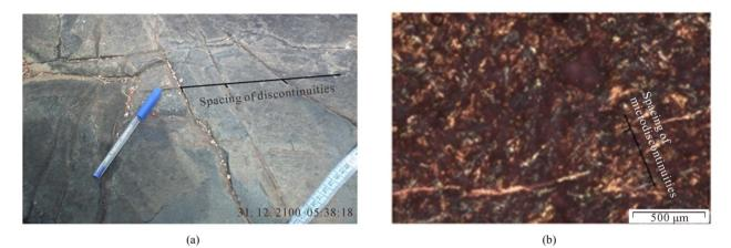
Figure 12. Fractal analysis of spacing of discontinuities ((a) outcrops scale; (b) preparation scale).
