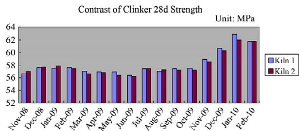
Figure 10. Contrast of clinker strength.
