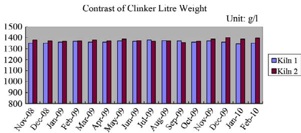
**Figure 11. Contrast of clinker litre weight.**
