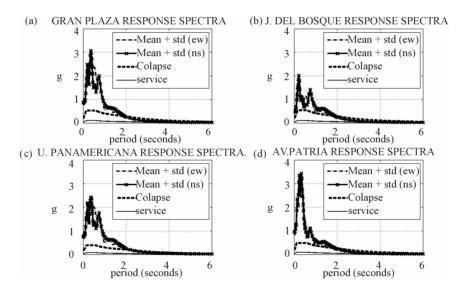
Figure 10. Response spectra calculated according to MOC-2008 procedure vs response spectra using seismic records. The different curves represent mean plus standard deviation response spectra for both components, response for a rock site, for edge state of service and for collapse. (a) Gran Plaza site; (b) Eulogio Parra site; (c) Av. Patria site; (d) U. Panamericana site.
