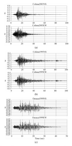
Figure 3. Horizontal acceleration records used. (a) Colima 2003 (Mw 7.5), (b) Colima 1995 (Mw 7.5), (c) Oaxaca 1999 (Mw 7.5).
