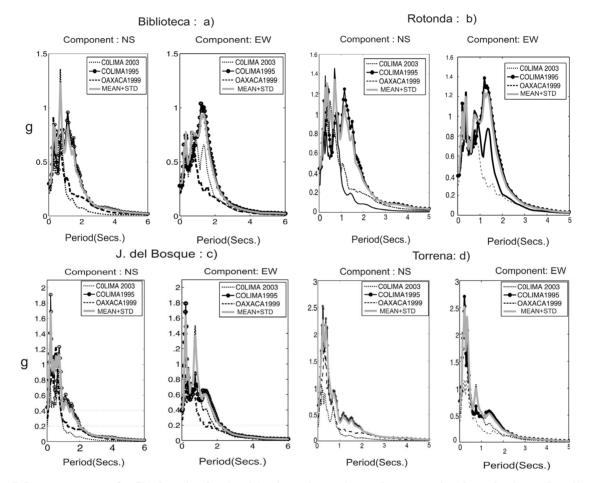
Figure 7. Response spectra for 5% damping for the eight sites using real records propagating through a layered media. Continuous line represents spectra using the Colima 2003 record, continuous line with dots, the spectra using Colima 1995 record, dotted line represents spectra from the Oaxaca 1999 record. Green line is the mean plus standard deviation. (a) Biblioteca site; (b) Rotonda site; (c) J. del bosque site; (d) Torrena site.
