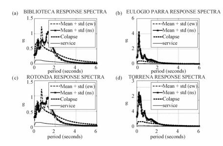
Figure 9. Response spectra calculated according to MOC-2008 procedure vs response spectra using seismic records. The different curves represent mean plus standard deviation response spectra for both components, response for a rock site, for edge state of service and for collapse. (a) Biblioteca site; (b) Rotonda site, (c) J. del bosque site; (d) Torrena site.
