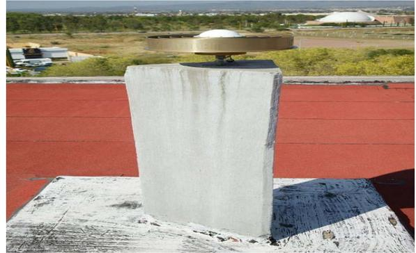
**Figure 2. Aguascalientes (INEG) station with choke-ring antenna, RGNA network. Date of photo February, 2000.**
