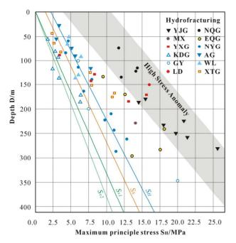
**Figure 2.** Vertical change of maximum principle stress in the Tibetan Plateau. Explanation:  $S_H$ , maximum principle stress of Yangbajain granite at NYG;  $S_h$ , minimal principle stress of Yangbajain granite at NYG;  $S_{v1}$  and  $S_{v2}$ , vertical stress caused by overlying rocks with average densities of 3.02 g/cm<sup>3</sup> and 2.7 g/cm<sup>3</sup> respectively. The shaded area refers to high stress zone for large earthquakes.
