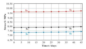
**Figure 4.** Diagram of stress changes in Northwestern Quxi granite. Explanation:  $S_1$ ,  $S_2$  and  $S_3$  represents piezomagnetic stress measured in bore hole at depth of 31 - 35 m at orientations of N40°W, S80°W and N20°, respectively, from January 13 to February 26, 2008.
