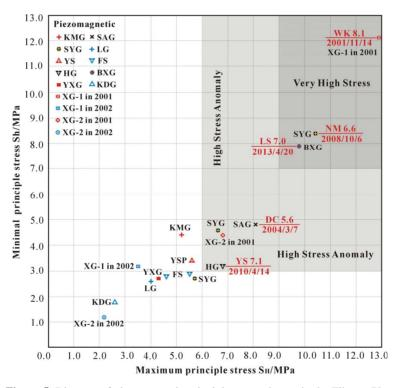
**Figure 5.** Diagram of piezomagnetic principle stress change in the Tibetan Plateau. Explanation: the SYG, KMG, FS and BXG *et al.* refer to the sites for piezomagnetic stress measurement, and the YS 7.1/2010/4/14 *et al.* refer to the related earthquakes occurred in recent years.
