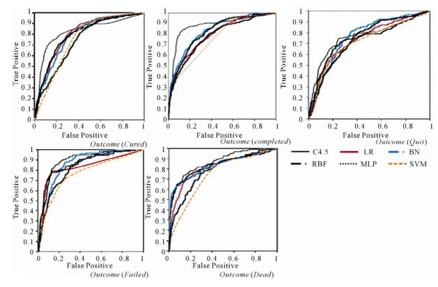
Figure 4. ROC curve for C4.5 decision tree, logistic regression (LR), Bayesian networks (BN), radial basis function (RBF), multilayer perceptron neural networks(MLP), and support vector machine on the task of classifying outcome of TB treatment course based on the target outcome including cured, completed, quit, failed, and dead. In all cases decision tree has outperformed other methods with area under curve 0.92 for cured, 0.94 for completed, 0.88 for quit, 0.96 for failed, and 0.85 for dead.
