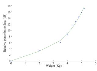
Figure 4. Response of grating to external applied pressure.
