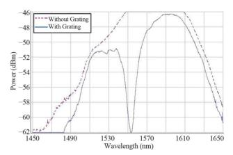
Figure 2. Spectral response of MLPFG in MSM fiber structure.
