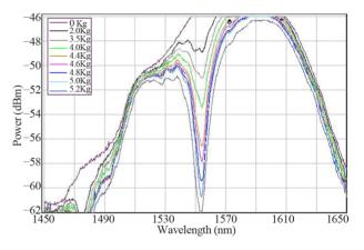
Figure 3. Complete transmission spectrum of MLPFG in MSM structure ( $\Lambda = 600 \ \mu$ m) with different pressures
